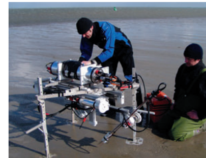
The instrument "Lance-A-Lot" maps structures at the sediment surface (e.g., ripples, mounds or pits) using a laser beam and a digital camera.
