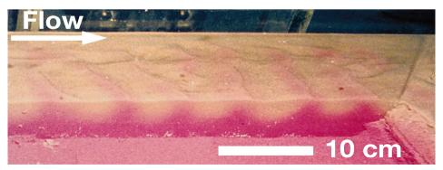
Fig. 1 Advective pore water transport in permeable sediment. Permeable sands exchange fluid and particles with the overlying water through advective pore water flows. In a laboratory experiment, red tracer dye shows the flushing of pore water from the sediment due to the advective pore water flows caused by unidirectional bottom flow (Photo by: M. Huettel).
