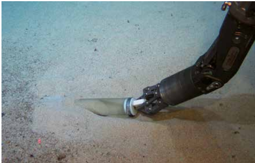
Fig. 3.31 ROV Kiel 6000 using a push corer to sample sediment on seamounts of the SW Indian Ridge.
