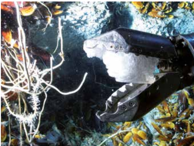
Fig. 3.11 ROV Victor 6000 holds a piece of gas hydrate which at certain temperature and pressure conditions, resembles ice. Atlantic Ocean, Gulf of Guinea.
