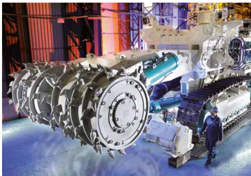
Fig. 1.11 Bulk Cutter (BC) built to be used for seabed mining. The machine is designed to cut material at high rates from seafloor massive sulfide deposits.
