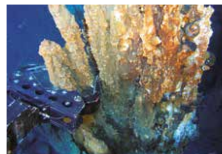
Fig. 2.2 Collecting samples from a deep-sea vent chimney using an ROV robotic arm.
