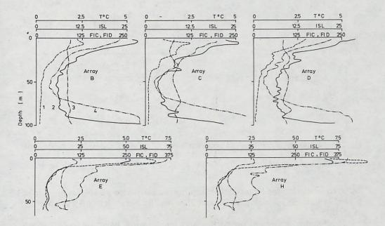
Fig. 1. Vertical profiles of mean values of FIC (1), ISL (2), FID (3) (in arbitrary units) and  $T^{\circ}C$  (4), calculated for the arrays B, C, D at station G-2, and E, H at station Z
