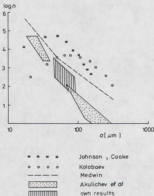
Fig. 8. Comparison of bubble concentrations obtained in various experiments in natural waters
