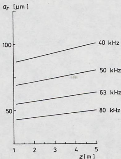
Fig. 2. Depth dependence of resonant bubble radius for frequencies used in the experiment
