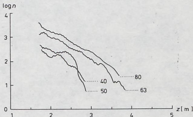
Fig. 6. Vertical profile of a resonant bubble number for frequencies 40, 50, 63, and 80 kHz
