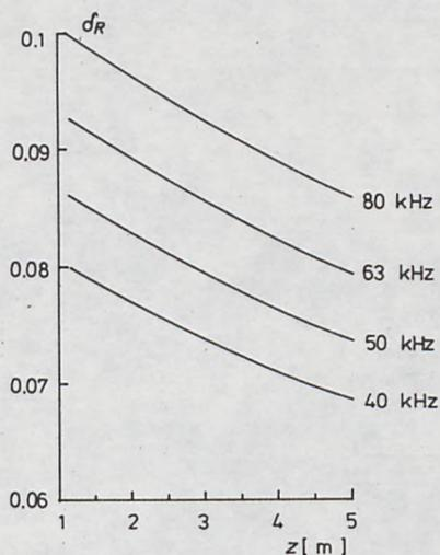
Fig. 5. Depth dependence of resonant damping constant for frequencies used in the experiment
