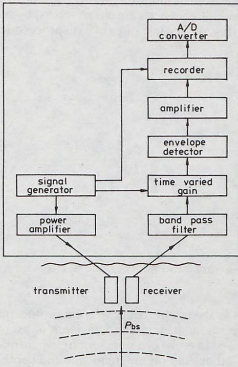
Fig. 3. Block diagram of the apparatus
