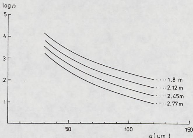
Fig. 7. Bubble size distribution for various depth levels
