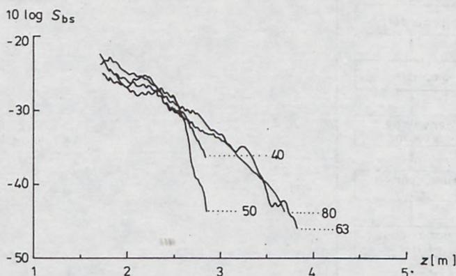
Fig. 4. Vertical profile of backscattering intensity for frequencies 40, 50, 63, and 80 kHz
