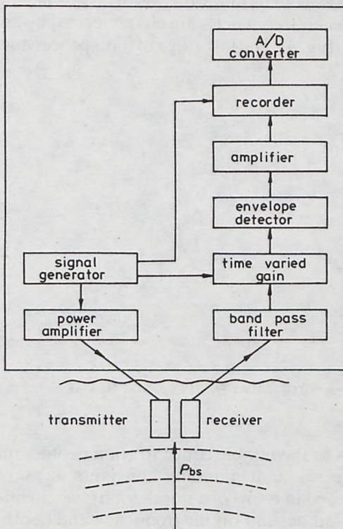
Fig. 3. Block diagram of the apparatus
