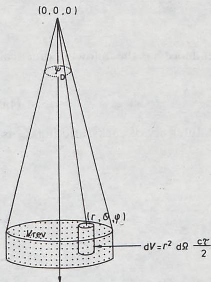
Fig. 1. General scheme of backscattering experiment
