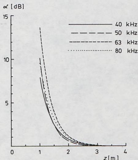
Fig. 9. Dependence of double distance attenuation on transducer immersion depth
