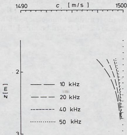
Fig. 10. Influence of bubbles on sound velocity in sea water
