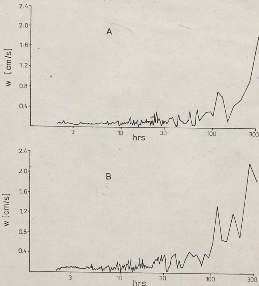
Fig. 8. Raw amplitude spectra of current velocity modulus in December 1980 and January 1981. A—station 2:  $N=1024$ ,  $Dt=1$  hr; B—station 3:  $N=1024$ ,  $Dt=1$  hr
