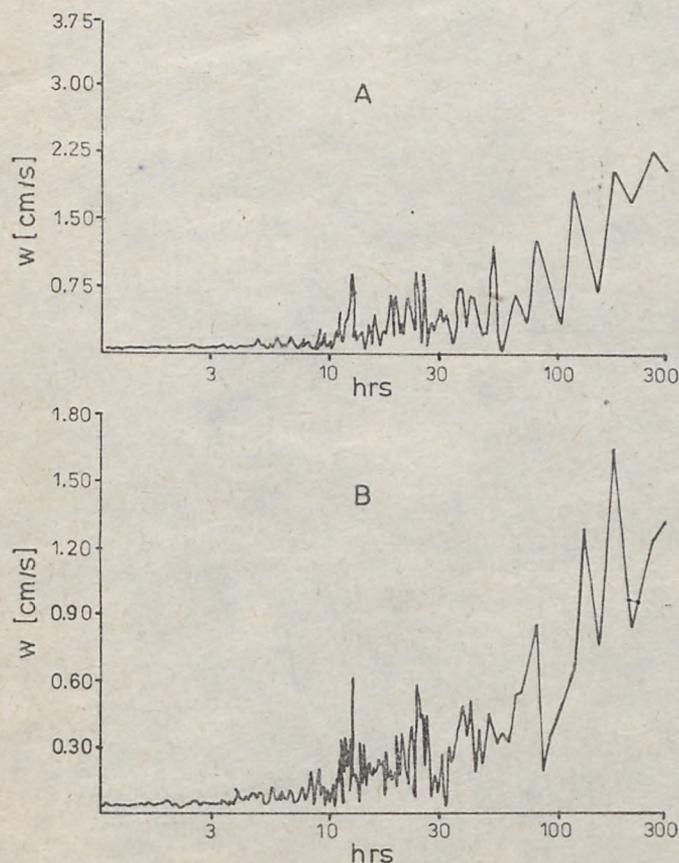
Fig. 7. Raw amplitude spectra of current velocity modulus in May and June 1980. A—station 1:  $N=2048$ ;  $Dt=05$  hr; B—station 2:  $N=2048$ ,  $Dt=05$  hr
