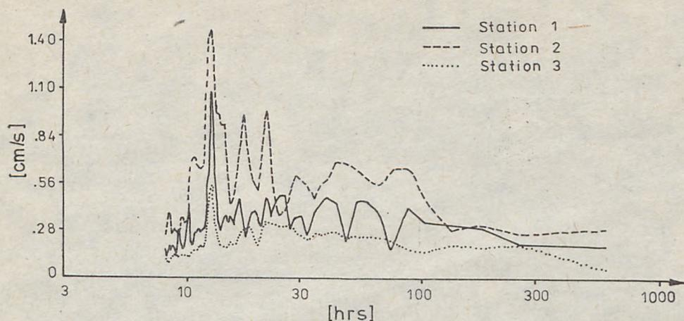
Fig. 12. Spectrum of averaged amplitudes for current along-shore component  $v$  (averaged for the whole period of measurements)
