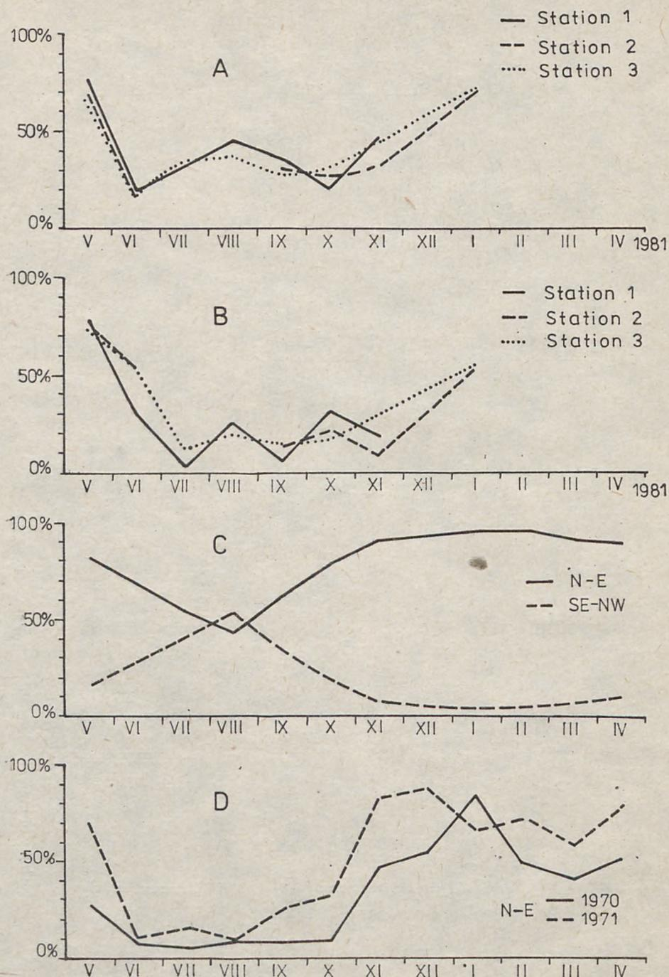
**Fig. 4.** Seasonal structure of current depending on trade-winds. A—percentage share of current direction in sector 165–195° in all observed directions; B—current stability [%]; C—percentage share of wind direction in sector N-E and SE-NW in all observed directions (for Nouakchott [9]); D—percentage share of wind direction in sector N-E in all observed directions (for Dakar [9])
