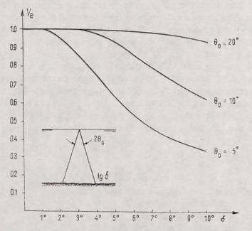
Fig. 1. Dependence of the measured coefficient of reflection from the bottom on the directional characteristics of the transmitting - receiving transducer and the inclination angle of irregularities of reflecting surface
