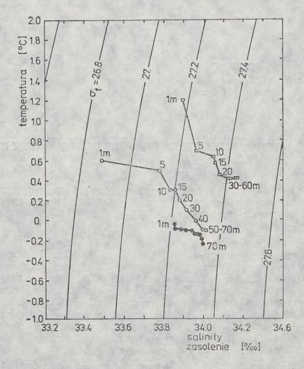
Fig. 1. T-S diagrams for Ezcurra Inlet waters with relative density isolines included  $\delta t$  (according to Dera [7])
