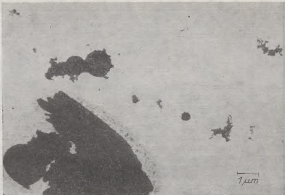
Photo 1. A micro-photograph of airborne aerosol particles on a ditizone-collodion film — a magnification of 9.600
