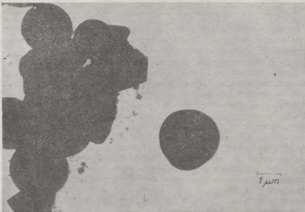
Photo 3. A micro-photograph of airborne aerosol particles on a ditizone-collodion film — a magnification of 9.600
