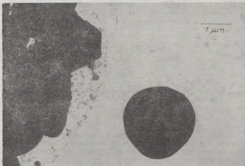
Photo 4. A micro-photograph of airborne aerosol particles on a ditizone-collodion film — a magnification of 15.200
